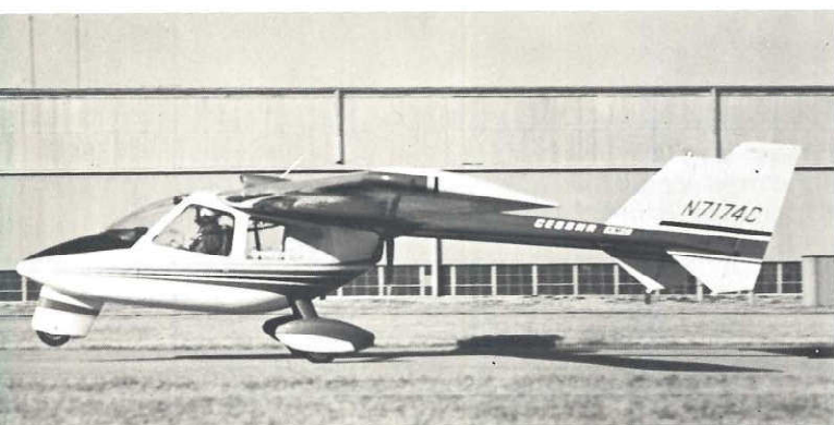
A new approach to light-plane design, Cessna's recently unveiled experimental XMC has twin tail booms, a slightly swept wing for better visibility, and a single engine behind the cabin.
